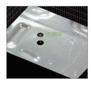
Hole positions and diameters can be measured accurately even for parts with complex shapes that cannot be laid horizontally.
