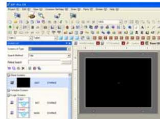
You can place switches or lamps on the screen by dragging and dropping contacts or coils on the logic program.
