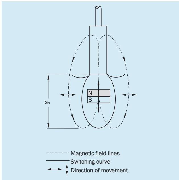
Case 2: The sensor responds if the magnet approaches the switching curve laterally. If the sensor leaves the switching curve, the sensor switches back again. This principle is largely used for magnetic cylinder sensors.
