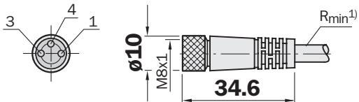
**Female connector M8, 3-pin, PUR halogen-free, angled**
