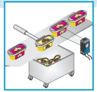
The label is on – but is it the right one? The CVS recognizes correct and incorrect labels by color.
