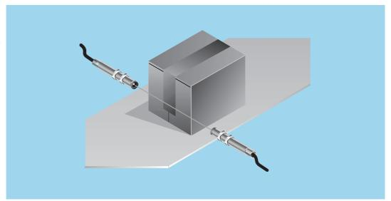
▼ VL 12 photoelectric reflex switches can also be used for the reliable detection of reflective surfaces, for example filmwrapped cardboard boxes.
